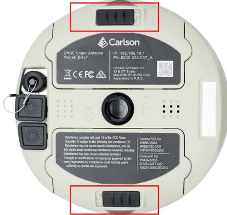
Figure 2-2: Battery latches
