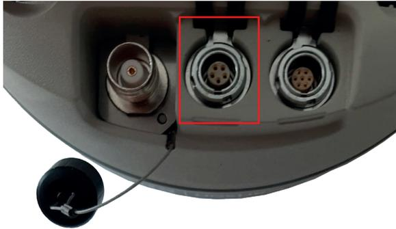
Figure 2-8: External power connector
