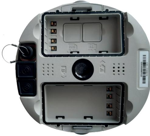
Figure 2-3: Battery compartment door removed
