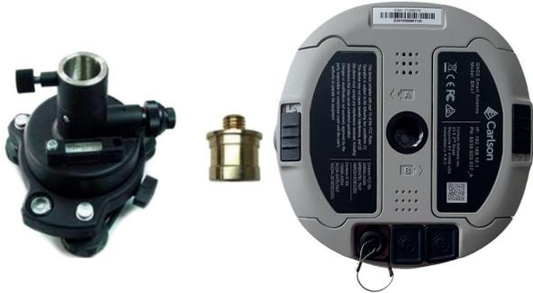
Figure 2-6: Installing BRx7 on a tribrach
