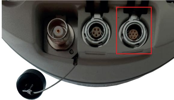
Figure 2-9: 7-pin diagnostic connector
