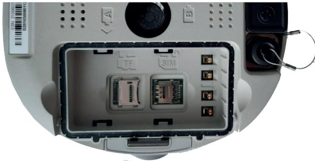
Figure 2-11: MicroSD/SIM card slot
