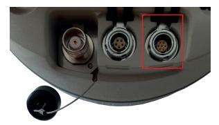
Figure 2-9: 7-pin diagnostic connector
