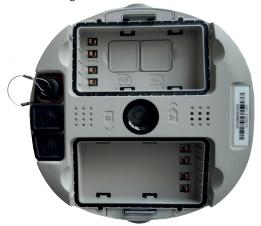
Figure 2-3: Battery compartment door removed
