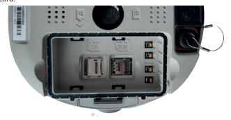
Figure 2-11: MicroSD/SIM card slot
