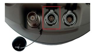
Figure 2-8: External power connector
