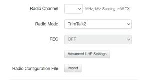
**Radio Channel:** Select a channel from the channel table provided by your dealer. The frequency, bandwidth, and transmit power (base only) is shown next to the channel.
