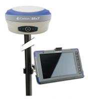
Figure 2-7: Range pole installation
